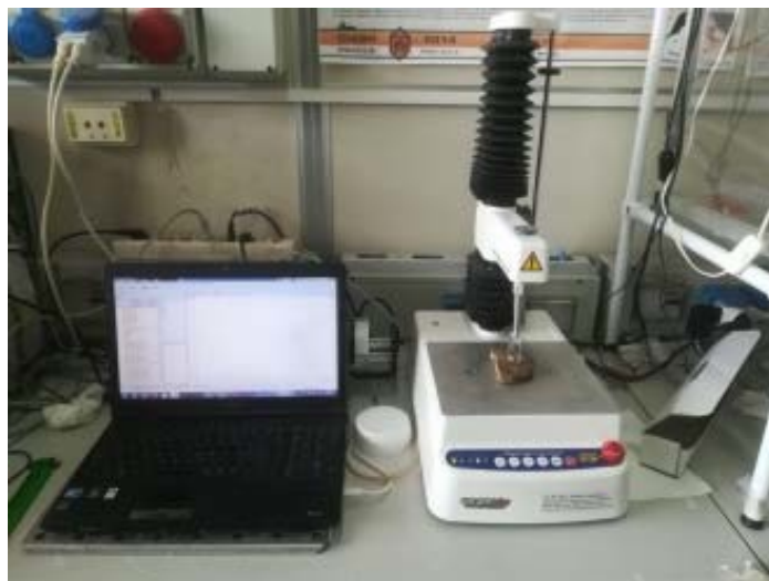
Figure 18. Hamburger subjected to compression test using the Texture Analyzer XT Plus.
